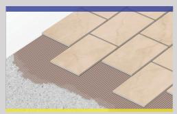
Install tiles in your preferred pattern. Complete grout application leaving grout lines clear as required. Use the Primer / Sealant on all porous tiles.
